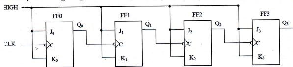
19. a. Give the function performed by the following circuit.
